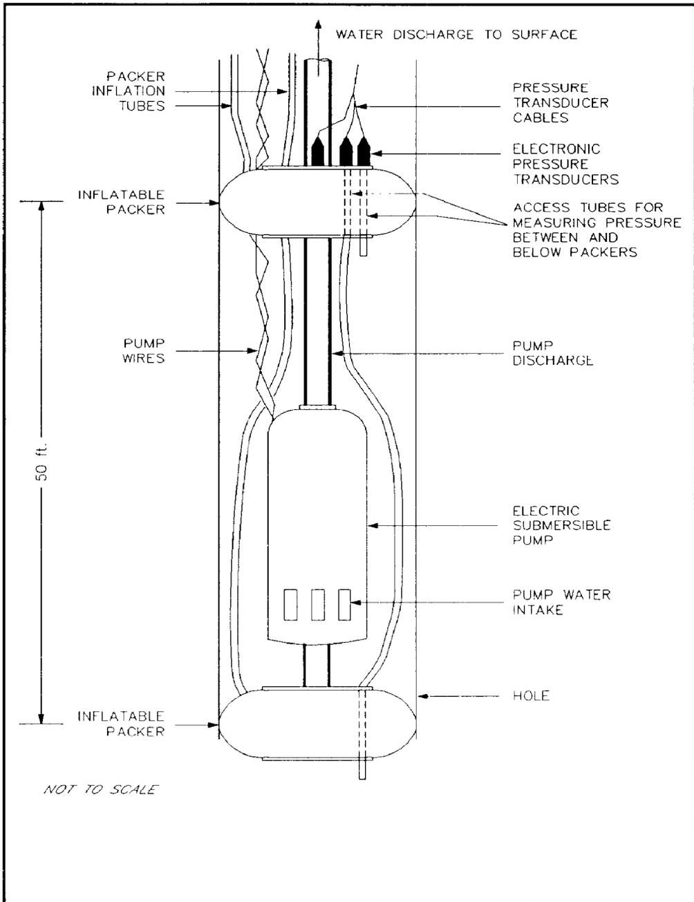
Fig. 2. Double inflatable packer/pump assembly.
